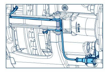
The new wear sensor assembly with code number 05.801.49.50.0 is downwards compatible and can be retro-fitted at any time; it supersedes the previous sensor assembly with code number 05.801.50.49.0.
