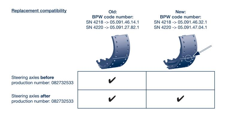
INST NB! ECO Drum brake shoes cannot be used with steering axles before production number 082732533.
