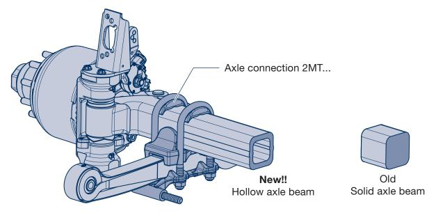
The release is valid for both positively steered and self-steering axles. It should be noted that the approval only applies to axles with 17.5" tyres (SN 3020) and in combination with the welded axle connection, called 2MT... (see figure).
