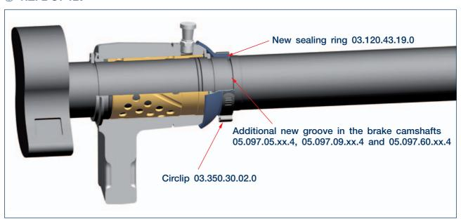
The introduction of the new additional groove will not result in a new code number; as a result the new sealing ring 03.120.43.19.0 can only be combined with the new brake camshafts.
