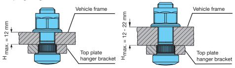
The hanger bracket is reinforced by a bracing plate directly by means of an attachment point on the head of the spring bolt. This means the forces are directly absorbed by the spring bolt. The stress on the hanger bracket and the bracing plate attachment is reduced and their service lives are improved. The bracing plate is not supplied by BPW.
