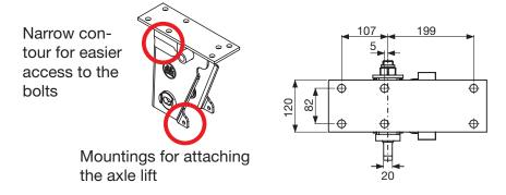
Top plate with hole pattern for attaching to the vehicle frame
