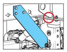
Special splined bolts are used for bolting the air suspension hanger bracket onto the vehicle frame. These grip the top plate of the hanger bracket preventing rotation and therefore can be installed very easily.
