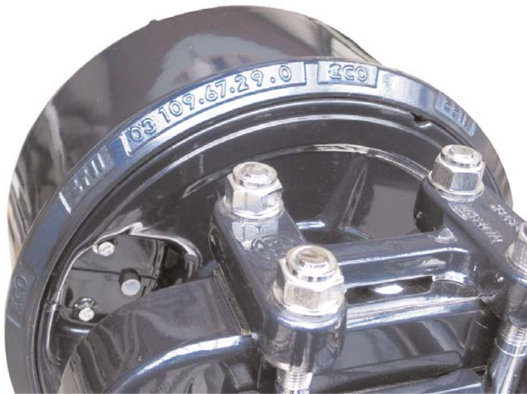
Fig. 1: ECO Drum drum-brake axle with Airlight II air suspension
