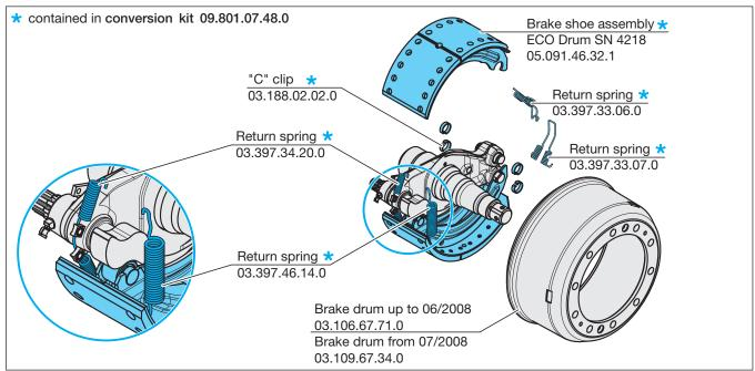
Previous axle beam versions (up to build year 06/2008) are retrofitted with ECO Drum brake shoes SN 4218 and the new return springs 03.397.34.20.0 and 03.397.46.14.0 when they come in for service. No groove is required in the brake anchor plate for the retrofit, because the middle part of the return spring 03.397.34.20.0 makes contact with the contour of the weld-on nuts and is therefore fully located.
