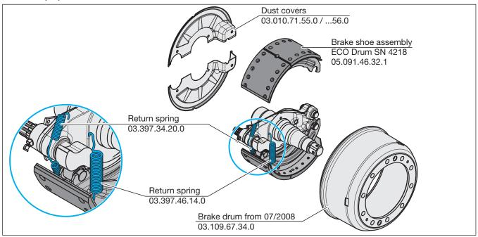
Positioning of one-piece return spring 03.397.34.20.0 on the outer contour of the brake mounting plate
