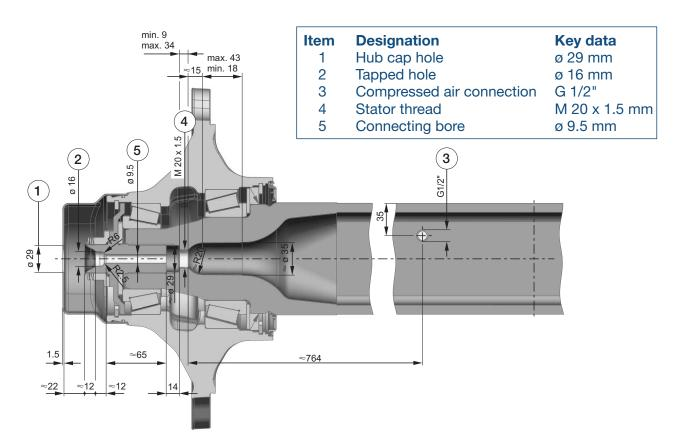
The axle is supplied with a standard hub cap to protect the bearing against moisture. The drilled hub cap intended for installation is also supplied as a separate item.
