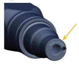
If the axle type plate becomes illegible, it is still possible to access the spare parts documentation by using the axle beam welding number.
