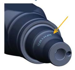
From June 2012, the axle beam welding number will now be stamped onto the axle stub on the front.
