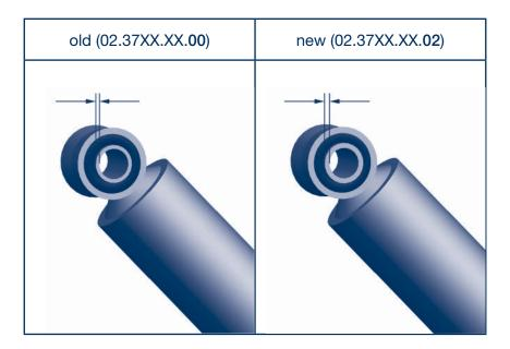
Attaching the shock absorber on the ECO Air COMPACT cast member now requires a higher torque than with the Airlight II designs. This means that reinforcing the bush is required.
