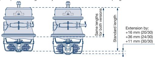
The DD standard cylinder can be replaced by the DD CCF cylinder depending on the installation space situation. The force output is within the tolerance range of the DD standard cylinder and is confirmed by a TÜV certificate; homologation is therefore not necessary.
