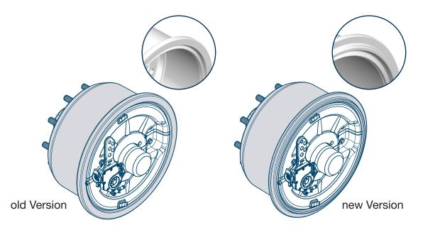
The further features of the ECO DRUM, such as quick and easy brake service thanks to the ECO principle and the particularly high-quality sealing of the brake camshaft bearing, are unchanged. With the series introduction of ECO Plus 3 bearing technology in 2023, BPW stub axles will also have an improved and wear-optimized wheel bearing seal and a new, remountable ABS exciter ring.
