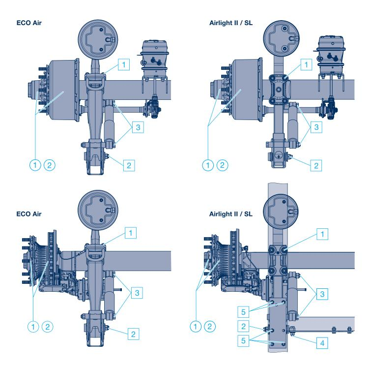
The Extended Warranty applies to the ECO hub unit, axle beam, trailing arm connection and hanger brackets. It is
