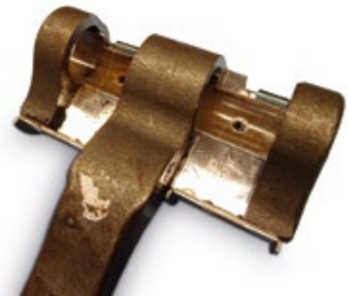
Original BPW brake lever after an endurance test
