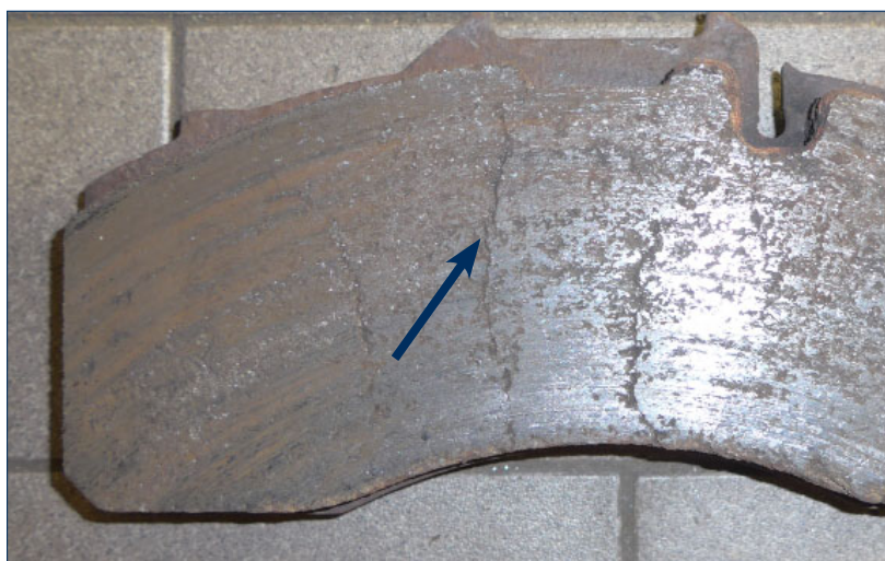
Figure 4: Cracks in the permissible area of the lining surface
