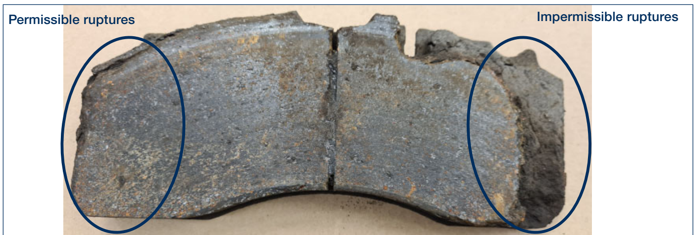
Figure 3: Lining with impermissible
