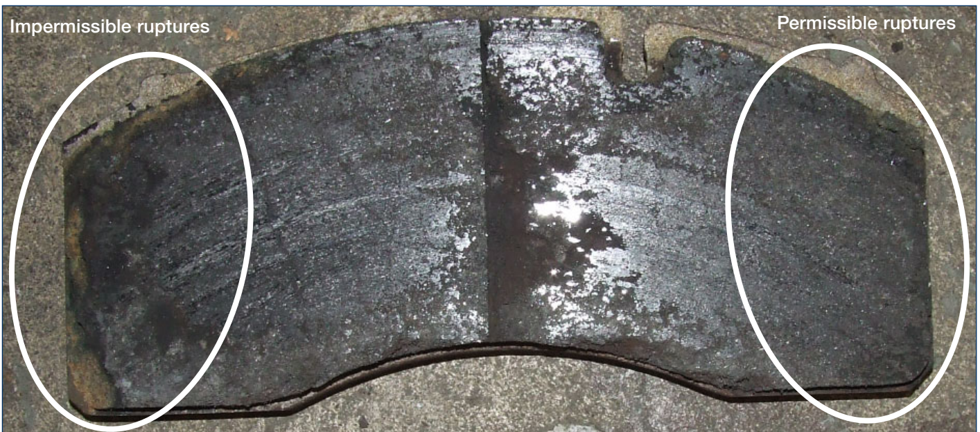
Figure 3: Lining with impermissible
