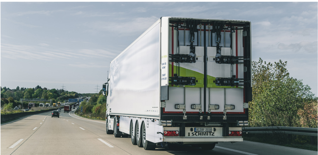
Improved aerodynamics reduces fuel consumption in semi-trailer trucks. Source: Betterflow. Source: Betterflow
