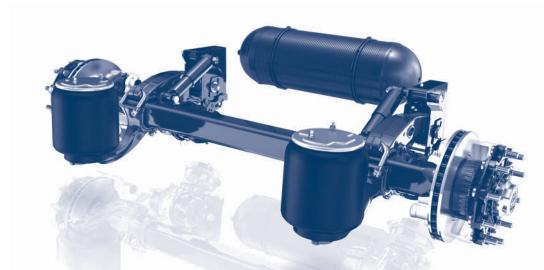
ECO Air COMPACT was developed for 9 tonne standard use with single tyres in on-road use and is available in the SN 4218 drum brake and also the TSB 3709 and TSB 4309 with 120 offset disc brakes brake versions.
