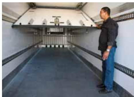
A collapsible moveable partition enables different temperature zones.
