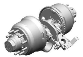
The integrated torque limitation also prevents incorrect operation when tightening and ensures that the bearing preload is at the optimum level. When the hub is pulled off, the taper roller bearings remain well protected against dirt and moisture in the hub. However, even if the bearings need to be renewed, this is possible without difficulty because DIN-ISO taper roller bearings are available worldwide.
