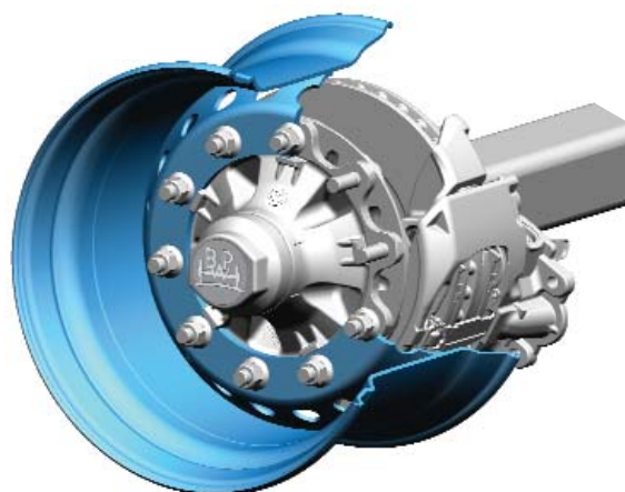
BPW rigid axle with Südrad no. SR 4070 (ET 0 = 0 offset).
