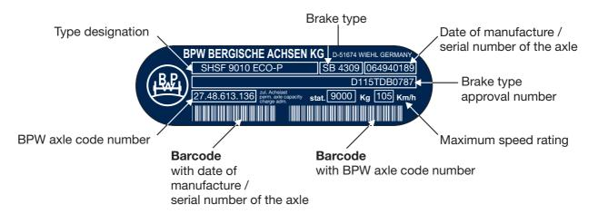
The BPW type plate will continue to be given a protective film. This film can then be removed when the painting process has been completed, so the lettering can remain legible. In addition to this, the BPW type plate has a strong adhesive laminate layer that provides permanent protection for its surface against damage.
