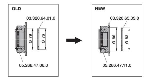
A different combination of axle nut and thrust washer as explained above is not permitted. Incorrect assembling may cause further damages!
